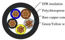
Polychloroprene rubber outer jacket Bare copper conductor Green/Yellow wire
